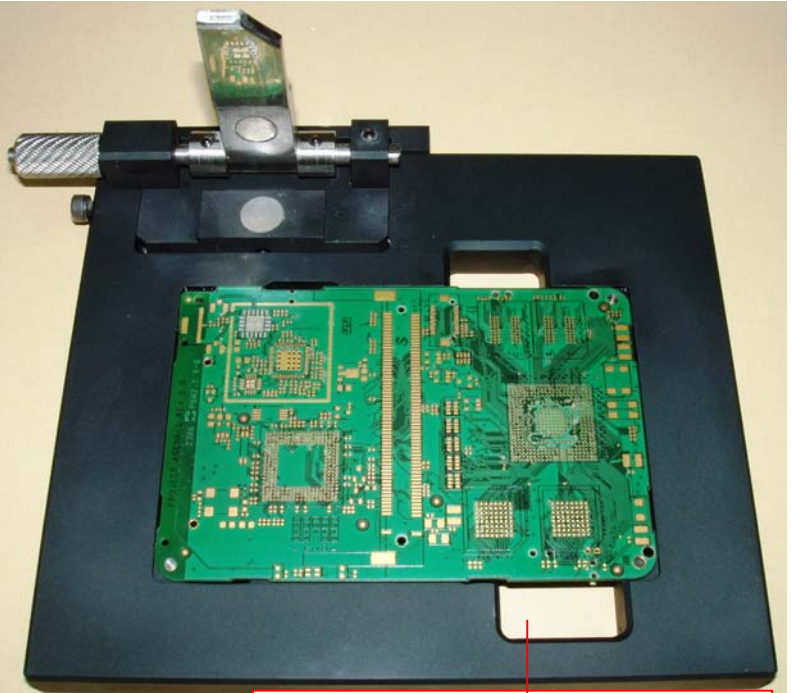
Cutout for ease in load & unload PCB
